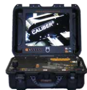
Portable Command & Control Unit (CCU)
