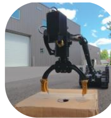
Box Opener Set of two blades on claw tips. Quickly opens boxes systematically.
