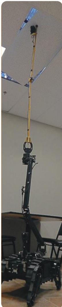
Camera Extension The camera extension is designed to access hard to reach places. The rubber tip is ideal for pushing through tiles, windows, and other obstacles.
