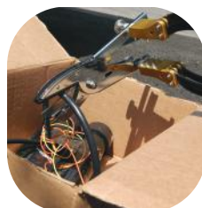
Wire Cutter Heavy Duty cutting tool that mounts firmly on Claw. Can be mounted on front or side Claw.
