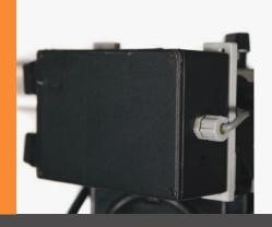
**Duke Pro Shock Tube Initiator** (P/N ESI-RM2-FLEX) Required for initiating the PAN disruptor or Bottle Charges and can be mounted on both the Claw arm and Weapons Arm.
