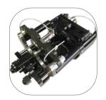
Twin 20mm Neutrex Mount w/ RAM (P/N 1400) Weapons turret head with integrated Recoil Absorption Mechanism (RAM). Holds two standard 20mm Neutrex disrupters. Disrupters not included. (Available for MK3 only)
