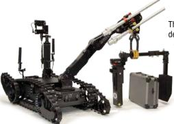
The OpenVision™ Integration Kit allows the OpenVision™ live video X-ray imaging system to be easily deployed remotely using the CALIBER® FLEX robot. The live video can be transmitted wirelessly and displayed on the robot's Command and Control Unit. (Open Vision™ live video X-ray imaging system not included).
