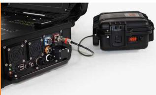
**CCU Battery Pack** (P/N CAL-DCPP)
