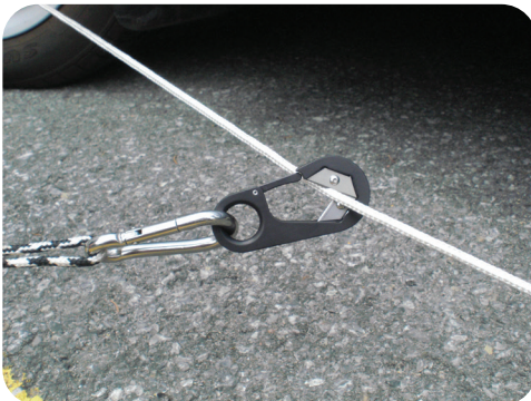
Pull line attached to CUTABINER®
