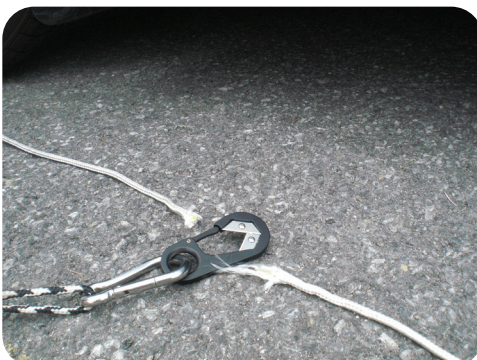
Pull line safely pulls CUTABINER® and cuts rope remotely
