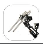
**Ideal Products PAN<sup>™</sup> Disrupter Unit** (P/N CAL-K100) 12 gauge, shock tube initiated disrupters. Recoil Reducer Kit is required to fire PAN<sup>™</sup> disrupters from the CALIBER® Robot. (Available for MK3 and T5)
