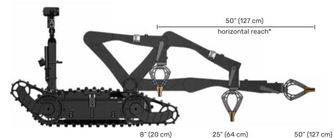
Maximum payload based on distance from chassis
