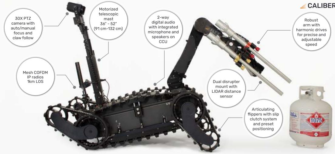
The operator can control the robot arm's elbow, shoulder and wrist simultaneously, making it easier to access tight and awkward spaces.
